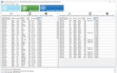
Figure 4.5: Code check results (worst utilization factors) reported in Sesam Wind Manager over all design load cases.
