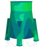
Figure 3.4: Results showing mesh with the stress distribution over the transition piece.
