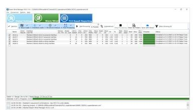
Figure 4.3: Sesam Wind Manager includes a grid to easily enter all design load cases for the analysis.
