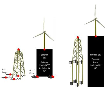
Figure 4.7: Various options for using seismic effects in a superelement analysis.
