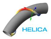
Helica performs short-term fatigue analyses based on histograms or time series imported directly from global analyses. Long-term fatigue damage is calculated by accumulating damage over all load conditions and directions. Helica also performs extreme load capacity checks in accordance with the ISO umbilical standard, and can calculate fatigue damage due to vortex-induced vibrations.
