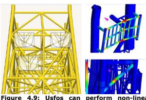
Figure 4.9: Usfos can perform non-linear analyses, such as boat impact analysis and push-over analysis.
