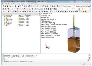
Figure 3.7: A jacket including wave and soil environment in GeniE.
