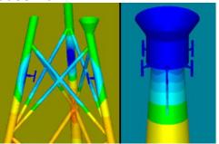
Figure 4.10: Surface corrosion potentials on a jacket and monopile.
