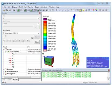
Figure 3.8: An example mode shape of a jacket structure visualized in Xtract.
