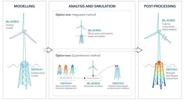
Figure 4.1: Industry workflows are supported – integrated and superelement.
