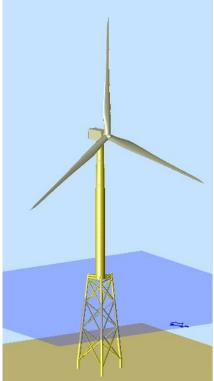
Figure 5.1: Combined turbine and support structure model in Bladed.
