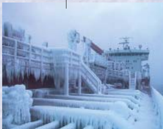
Ice formation on the deck, superstructure and cargo threatens both the performance of deck equipment and the vessel's stability.
