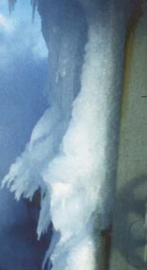
Ice formation on the deck, superstructure and cargo threatens both the performance of deck equipment and the vessel's stability.
